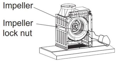
6. Clean the impeller and volute inside and outside with a soft brush with neutral detergent and then install it in reverse order.
