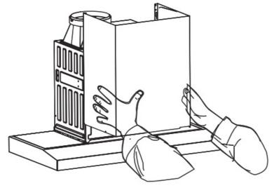
3. Remove the screws on the frame cover and remove the frame cover.
