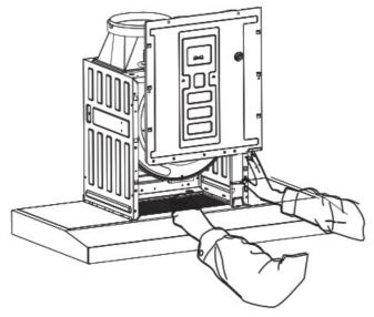
4. Remove the screw from the volute and the nozzle and remove the inlet wind ring.
