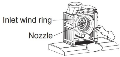
5. Turn the lock nut and remove the impeller in the direction of the motor shaft.
