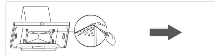
1. Hold the mesh by hand, use the cross screwdriver to top the filter to the left and right sides of the filter, open the screen.
