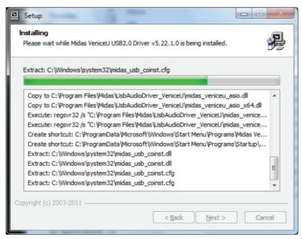
6. During the installation procedure, the following dialog box will appear. Plug the USB cable into the VeniceU console (type B connector) and into your PC (type A connector). Then switch on the console and click OK in the dialog box.
