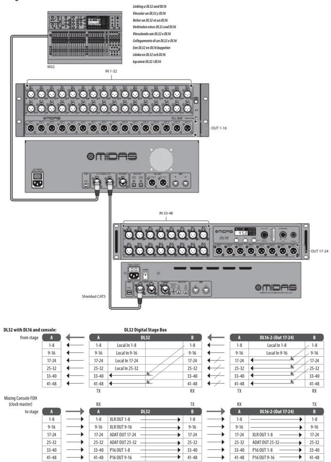
Note: The signals on both units are fully defined on the M32's 'Routing/AES50 Output' page.
