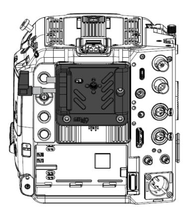
• For the Remote Start / Stop function (R/S), install a 2.5mm TRS Cable into the DB-10 REMOTE port.
