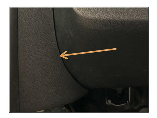
• Using a pry tool remove intermediate panel between A pillar and kick panel
