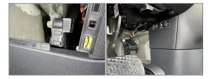
Reconnect battery disconnect cable from to post from step 2
