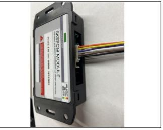
The SKSNG907 and SKSNG907RV with software version 5.26 and up include a 6 pin expansion port and pigtail. This is a 6 wire pigtail with a white plug. The gray wire is used for hood pin (required), as covered in step 20. With this port, you can also add optional expansions:
