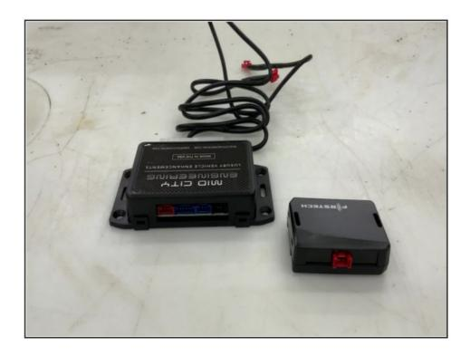
To install optional Compustar DAS sensor, connect data cable from DAS sensor to red port labeled Sensor on module labeled SmartKey Starter
