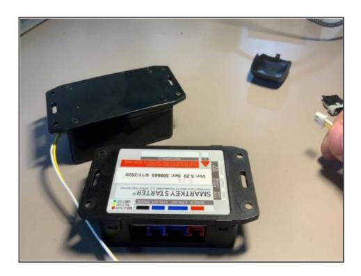
• Connect the 2 pin white plug from the key box to the 2 pin white port labeled 'KEY' on the module labeled 'SmartKey Starter'
