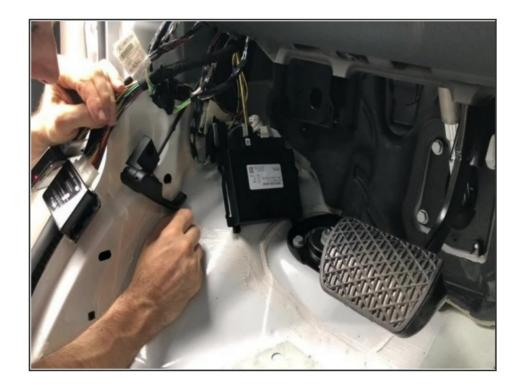
• Place and clip PCM module back into bracket
