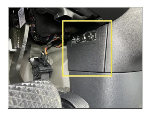
There is a battery quick disconnect that should be used to disconnect the chassis battery ground before performing this bypass
