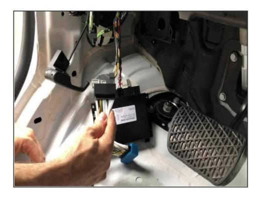
• Connect and latch 32 pin black plug from T-harness into PCM module where plug was removed in last step
