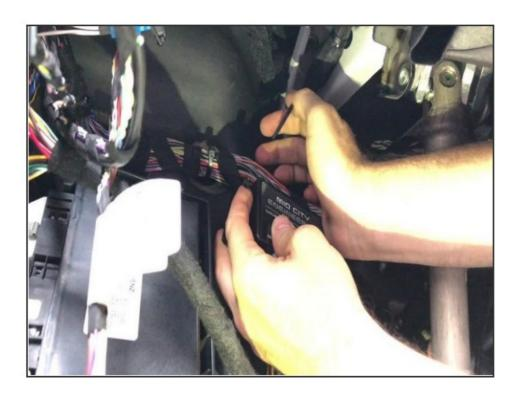
• Mount SmartKey Starter® and SKSPCM module in secure location. Suggested location is to wiring harness in driver under dash additional key security
