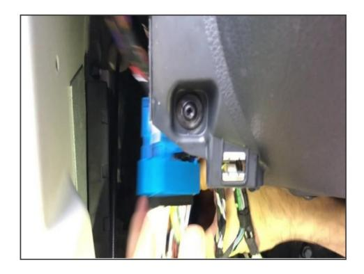
• Connect and latch blue or red 32 pin connector from T-harness to top of EIS module where plug was removed in previous step
