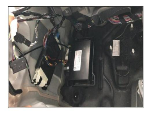
• Un-clip PCM module from bracket in back of kick area (towards driver front tire)
