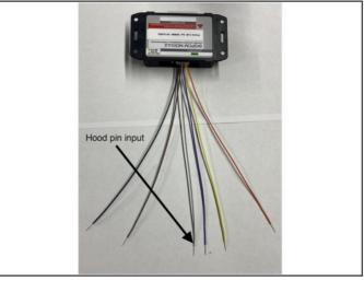
ARun wire from hood pin securely through firewall and run to driver side under dash area
