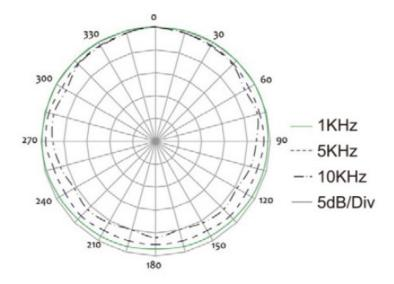
The i437C is an Omnidirectional microphone.
