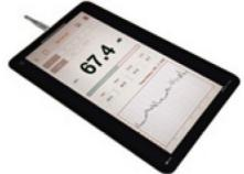
By pairing the i437C (or i437L) microphone with the Noiselab App from Apple Store, the iPad Pro can be used as a professional sound level meter, and it has passed IEC 61672-3 Class 2 requirements.
