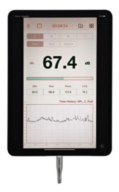
Simply plug the i437C microphone into the Type-C connector of iPad Pro (or other Apple products with a Type-C connector). Please note that i437C microphones DO NOT work with Android devices.
