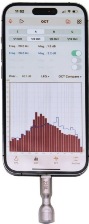
i236L matched with NoiseLab software on iPhone 14 Pro.
