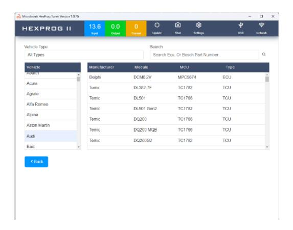
HexProg II Tuner software offers convenient ECU search options by part number and ECU name, facilitating easy browsing by list or car. This is especially useful for Bosch ECUs without labeled names, but only part numbers. The software also allows manual selection of specific ECUs from manufacturers, providing flexibility in tuning.
