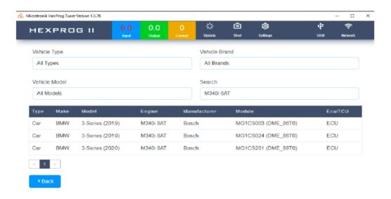
After selecting a vehicle, users will be directed to a page displaying all pertinent details such as the model, engine type, and year of manufacture. This allows users to verify that the information matches their own car model. Once they have confirmed the accuracy of the details, they can proceed to the ECU/TCU read/write option.
