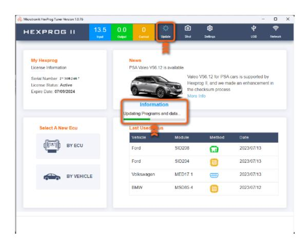
The update button is given on the home page in between the voltage/current display and the screenshot button. HexProg II Tuner software has a convenient update button on its home page. This button turns orange when a new version is released. Users can simply click the update button to install the latest version, which brings new features and supports additional ECUs.
