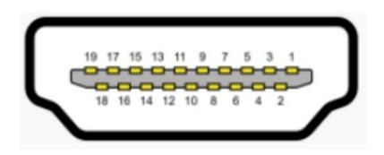
The video signal input via HDMI female connector. Connector Pin Assignment:
