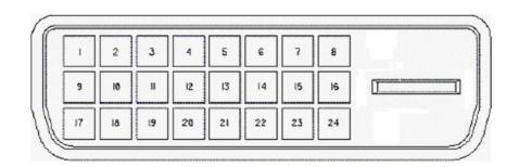
The video signal input via DVI female connector. Connector Pin Assignment:
