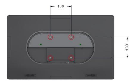
The monitor may be mounted horizontally (output connectors facing down) or vertically (output connectors facing right). Ensure that the surface material and the standard VESA wall mount bracket (purchased separately) are strong enough to support the weight of the monitor (refer to the Specifications table below for weight information). To maintain proper ventilation and heat dissipation, keep at least 60mm of clear space from the mounted display to the mounting surface.
