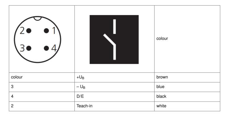
Fig. 1: Pin assignment with view onto sensor plug and colour coding of the microsonic connection cables
