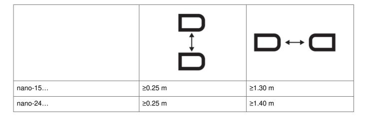
Fig. 2: Minimal assembly distances
