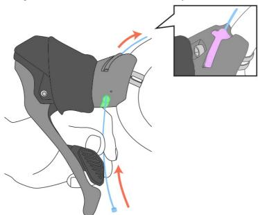
Install a housing cap on the end of your remote housing. Slide the housing around the cable and seat the cap in the housing stop on top of theshifter. Follow your frame manufacturer's guidelines for proper dropper cable routing and connect the cable to your dropper post according to the manufacturer's guidelines.
