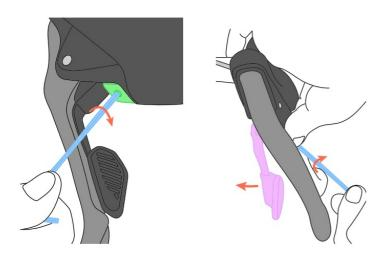
Unthread the cable set screw with a 2mm hex wrench one full turn. This allows the lever to return to the riding position.
