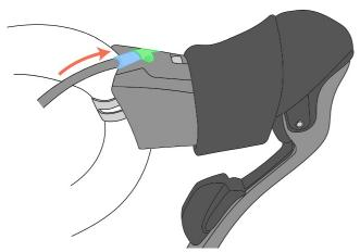
Test the dropper for full function by actuating the lever.
