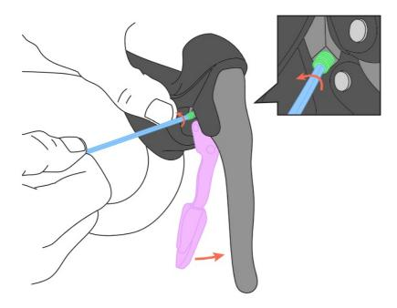
When the lever returns to the riding position, tighten the cable set screw with a 2mm hex wrench. Tighten until Snug. If the cable set screw is not snug, the remote lever will not engage the cable and the dropper post will not actuate.
