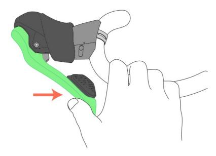
Pass the brake cable through the cable head seat inside the lever body and make sure the head of the cable fully seats in the lever body.
