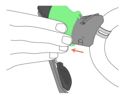
Route the cable through the cable port on the lever body and out through the top of the shifter.
