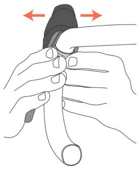
Torque the **band clamp** to **8Nm** and roll the hood back into place.
