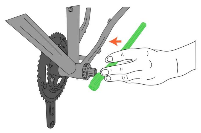
4. The crank includes a washer that goes on the preload bolt. Make sure the washer washer is on the preload bolt.
