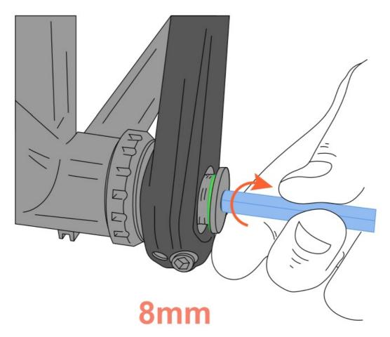
6. The preload bolt is for removing play between the spindle and bottom bracket bearings. Lightly tighten the preload bolt until there is no play between the spindle and bottom bracket bearings and no further, about 1-3Nm.Check for play by rocking the crank arms side to side. If play exists, tighten the preload bolt further. Do not exceed 3Nm.
