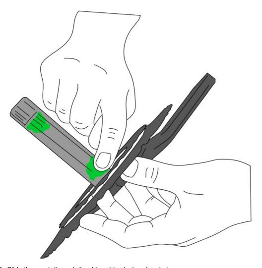
2. Slide the crank through the drive sidev bottom bracket.
