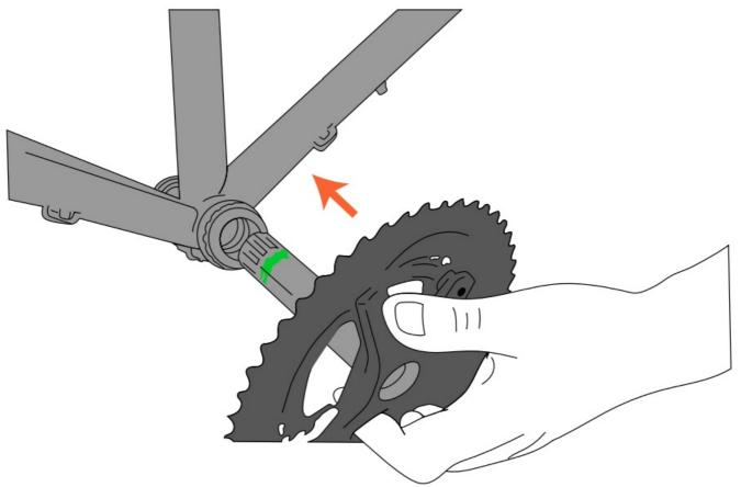
3. Slide the left side crank arm onto the spindle.
