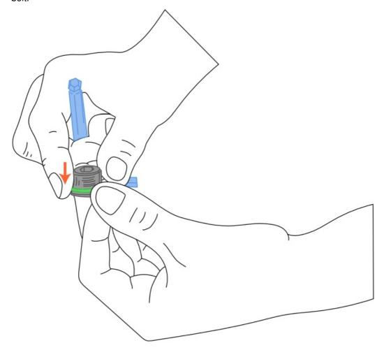
5. Thread the preload bolt into the spindle with your 8mm hex wrench.
