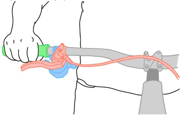
Put your hand in your normal riding position. With your index finger on the brake lever, test out the shifter position of both the upper shift lever and lower shift lever with your thumb. You should be able to reach both levers easily without losing your grip. Repeat step 3 & 4 until the setup is comfortable.
