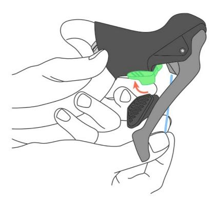
A clockwise adjustment moves the large paddle towards the handlebar and a counterclockwise adjustment moves the paddle away.
