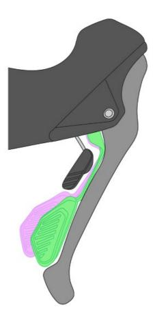
Move the small paddle out of the way and use a 1.5mm hex wrench to adjust the movement of the larger shift paddle.
