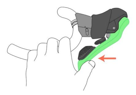
Pass the brake cable through the cable head seat inside the lever body and make sure the head of the cable fully seats in the lever body.
