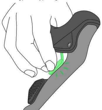
Roll the hood on the shifter towards the brake lever.
