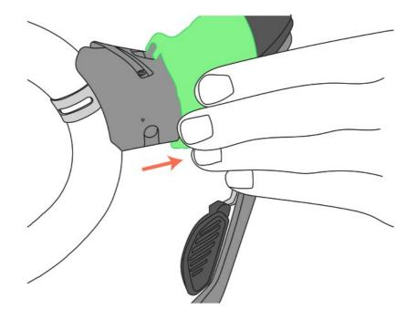
Route the cable through the cable port on the lever body and out through the top of the shifter. Pull tight to make sure the cable head is fully seated in the shifter.
