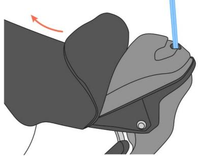
A clockwise adjustment move the lever towards the handlebar. And counterclockwise adjustment moves the lever away from the handlebar.
