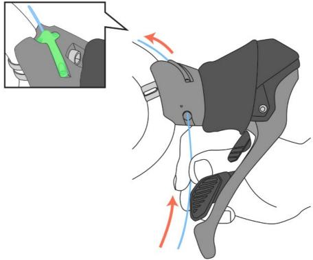
Install a housing cap on the end of your shift housing. Slide the housing around the cable and seat the cap in the housing stop on top of the shifter. Follow your frame manufacturer's guidelines for proper shift cable routing.
