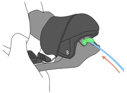
Seat the cable housing in the back side of the lever body.
