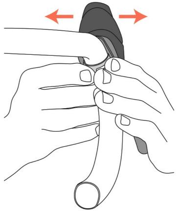
Torque the band clamp to 8Nm and roll the hood back into place.
