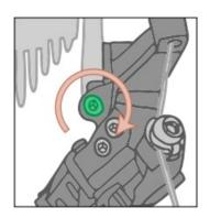
Snap the derailleur adjustment tool on to the guide pulley. Make sure the tool is touching the chain but not touching the cassette cog. Tighten the B-tension screw if the tool does not have enough room.
