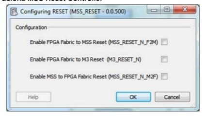
The reset controller manages the SmartFusion2 MSS reset resources. For complete details please refer to the Microsemi SmartFusion2 User's Guide.
