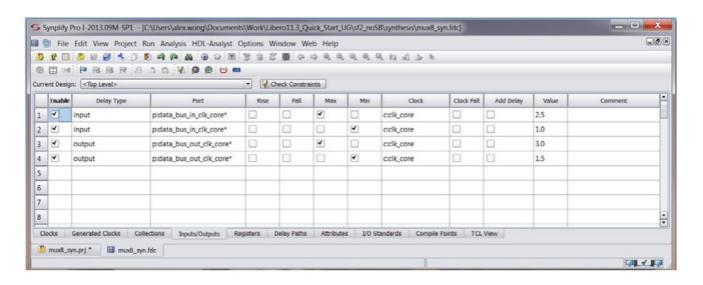
Figure 2-6 • Inputs/Outputs Tab
