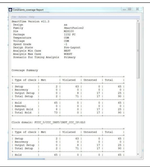
Figure 2-9 • Constraint Coverage Report
