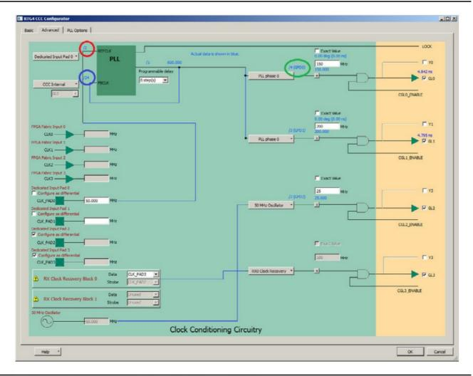
Figure 3-3 • RTG4 Fabric CCC Configurator (Advanced Tab)
