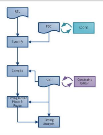
Figure 2-1 • Timing Constraints in the Design Flow
