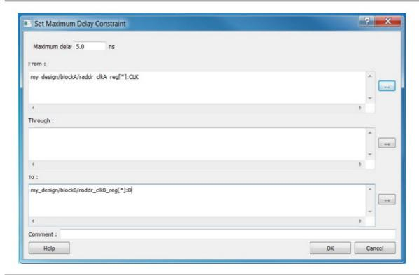
Figure 2-11 • Set\_max\_delay Constraints in Cloned Scenario
