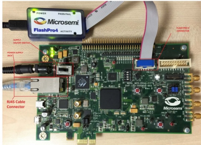
Figure 7 • SmartFusion2 Security Evaluation Kit Setup
