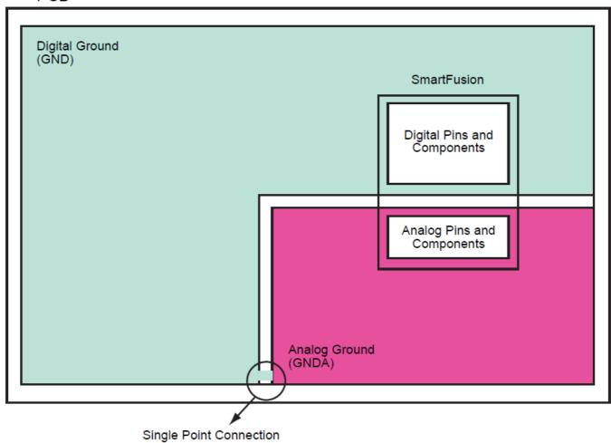
In complicated system designs and more complicated device packages, the placement of a SmartFusion cSoC device may not be as straight forward as shown in the simplified diagram of Figure 2. However, in any board layout, it is critical to keep digital signals and their return paths well isolated from the analog domain. The "Isolation of Ground Planes" section discusses an example of SmartFusion cSoC device placement and ground plane layout in a real-world mixed signal system design.
