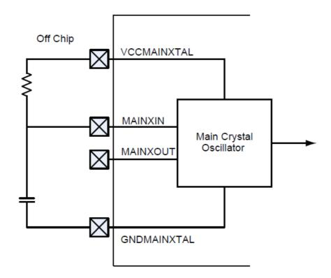
The frequency generated by the circuit in RC Network mode is determined by the RC time constant of the selected components, as shown in Figure 7.
