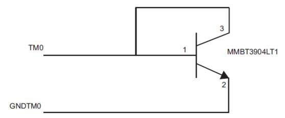
**Scenario 2:** When both TM0 and TM1 are used for temperature measurement. In this case, the connections are done with the GNDTM0 being connected as a common return path for both TM0 and TM1 as shown in Figure 14.
