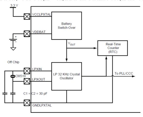
VCCLPXTAL is connected to 3.3 V and GNDLPXTAL is connected to ground in this mode. VCCLPXTAL supplies power to VRPSM block. Hence it must not be grounded, even if the low-power crystal oscillator is not used. The 32 KHz low-power crystal oscillator and the real-time counter (RTC) can be powered externally by a CR2032 type of lithium coin cell. As seen in Figure 9, a battery switch-over circuit is integrated into the SmartFusion cSoC
