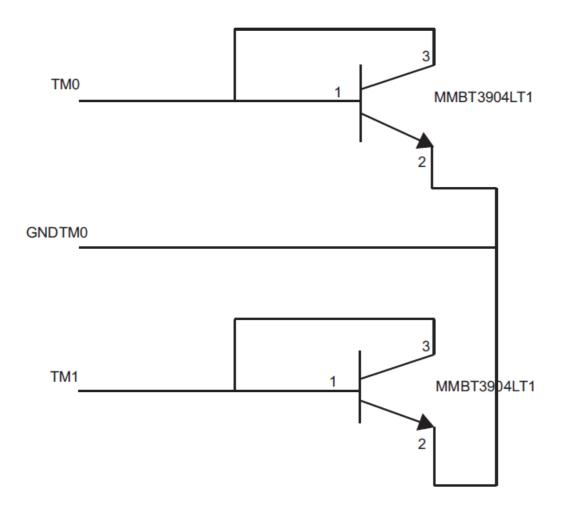
**Scenario 3:** When both TM0 and TM1 are used for direct current measurement or not used at all. In either case the GNDTMx pin can be left floating. If temperature monitor is not used, the ADC multiplexer (MUX) will not select the internal temperature monitor output (the internal TM[n] opamp output) to the input of the ADC. For this reason, whatever the TM input be, it will not be sampled by the ADC, but will only sample what the TM pin is configured to.
