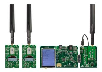
The plug-and-play LoRaWAN test kit provides a quick and easy operation of Micropelt's MLR003 radiator valve actuator together with a temperature sensor.
