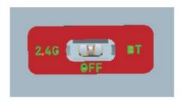
When the fluctuation switch is set to 2.4G position, it is 2.4G mode, when it is set to BT, it is Bluetooth mode, when it is set to OFF, turn off the battery power, plug in the USB cable for wired mode test.
