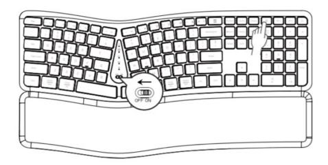
**Step 3:** Remove the USB receiver from the buttom of the keyboard and insert it into your device. Wait for 1-3 seconds to connect successfully.
