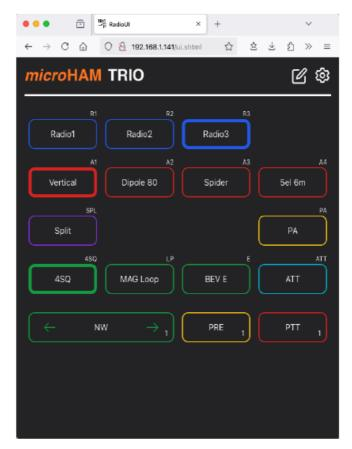
Web UI provides all buttons available on the controller front panel, including RX
