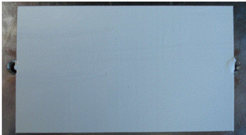
Figure 2-1. Grease on the Heat Sink Before Assembly
