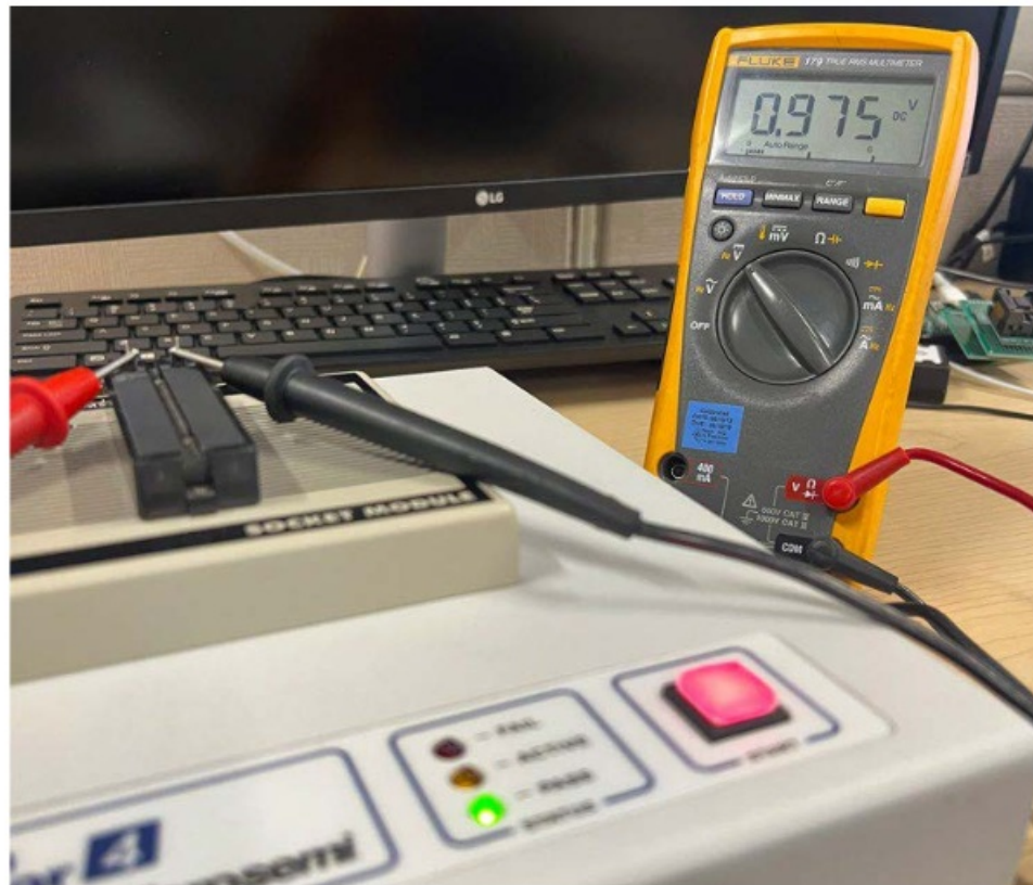
Figure 9. Voltage Measurement of the Pin 1
