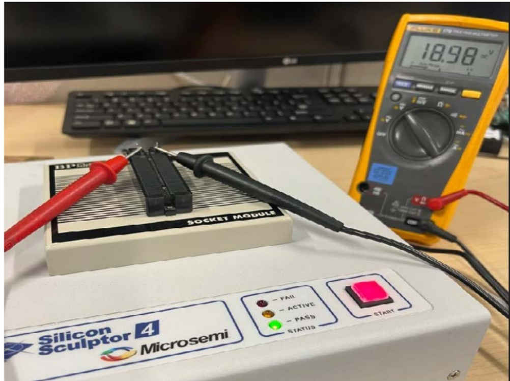
Figure 7. Voltage Measurement of the Pin 1
