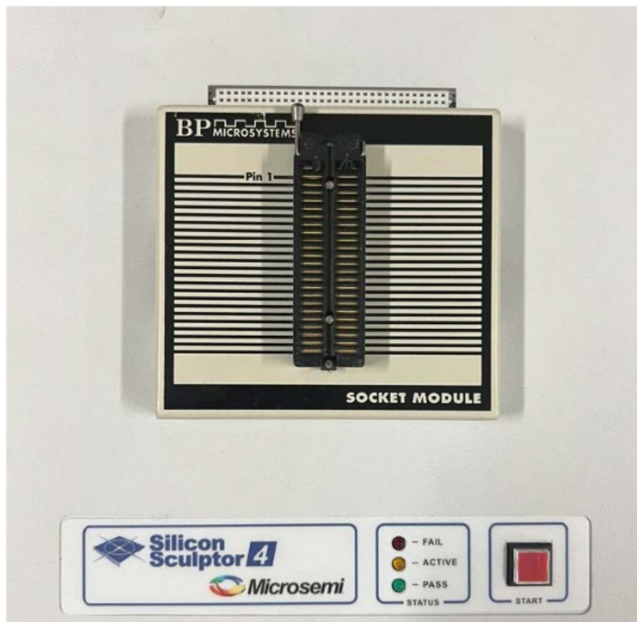
Figure 2. SM48D/SM48DB Socket Module Placed on SS4 Programmer
