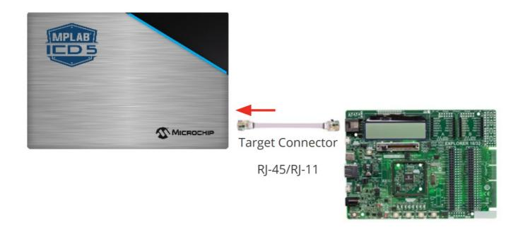
\*External target board power supply provided by user.
