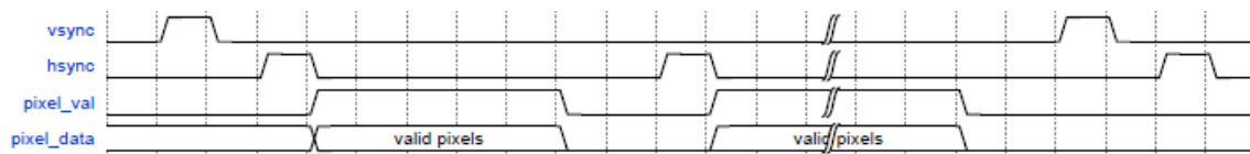
Figure 4-1. Timing Diagram for Output Video Stream Interface Signal
