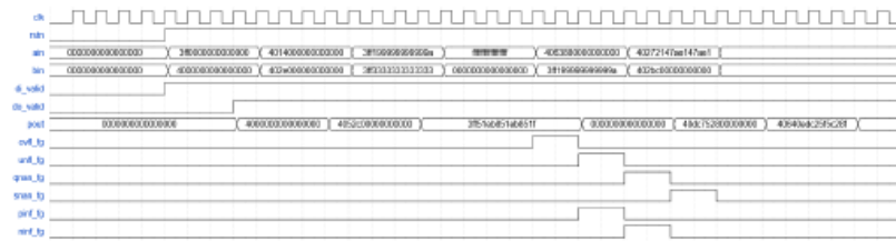
Figure 4-15. Floating-Point Multiplication (64-bit)
