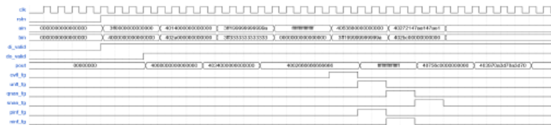
Figure 4-12. Floating-Point Subtraction (32-bit)
