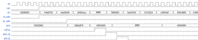
Figure 4-9. Floating-Point to Fixed-Point Conversion (64-bit)
