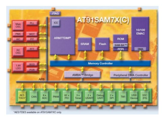
The AT91SAM7X(C)512B family are both sourced from the same wafer mask set. This design has a mask level
