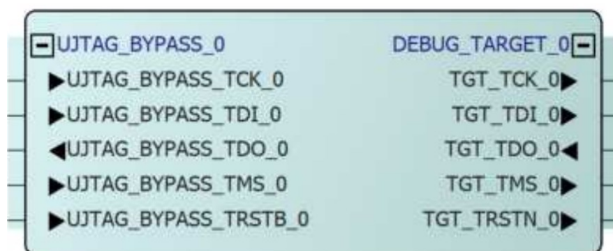
Figure 4-2. SmartDesign CoreJTAGDebug Instance using GPIO Pins
