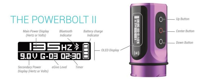
**Battery Charge:** 4 bars = 100%, 3 bars = 75%, 2 bars = 50% and 1 bar = 25%. Single bar will blink to indicate when there is aproximately 5 minutes left of operation. **Note:** Screen will switch to sleep mode after 15 seconds when device not in use. Press the power button to wake.
