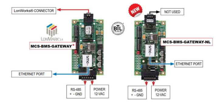
MCS-BMS-GATEWAY-NL units have the following 2 ports: RS-485 + Ethernet MCS-BMS-GATEWAY units have the following 3 ports: LonWorks® + RS-485 + Ethernet \*MCS-BMS-GATEWAY with LonWorks® is currently on backorder due to supply limits.
