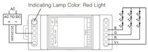
4. Controller connect to RGBW LED strip diagram
