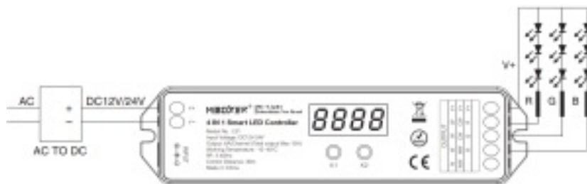
Controller connect to RGB LED strip diagram
