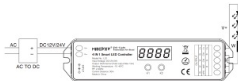
Controller connect to Single Color LED strip diagram
