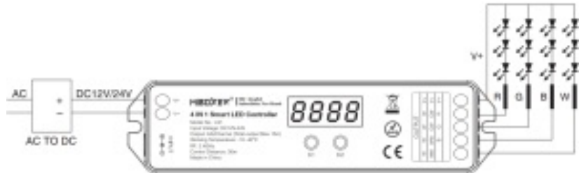
Controller connect to RGBW LED strip diagram
