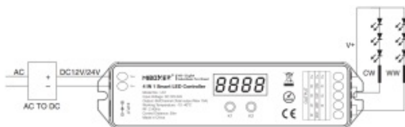
Controller connect to CCT LED strip diagram
