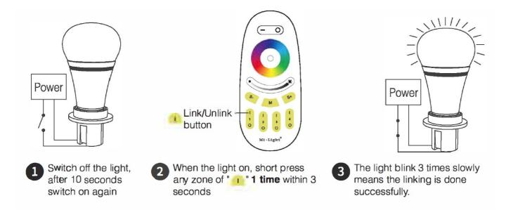
• A\ If the light does not blink slowly, the linking failed, Pis switches off the light again, and follows the above steps again.
