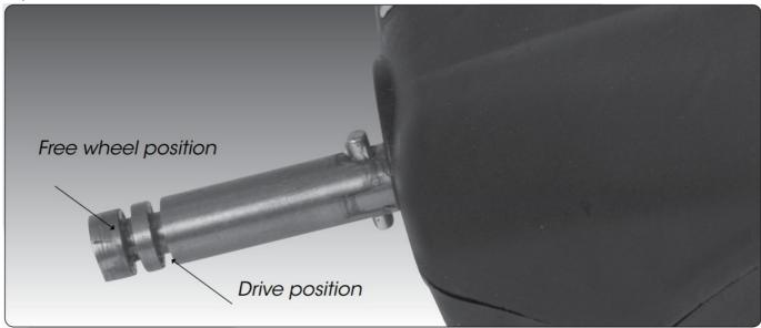
i. Drive position – Lock the wheel onto the groove closest to the battery base. To do this, press the grey release button on the wheel hub, push the wheel on to the axle as far as possible. To test for drive position try rolling the wheel backwards. If you feel resistance then the wheel is now in drive position and ready to use. Repeat for other wheel.
