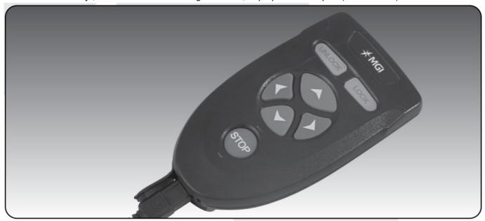
To check the level of power in the remote, press any button to signal the digital top box and the remote control battery level will show on the screen of the Zip Navigator.
