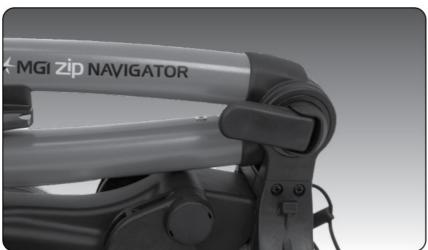
Step 6: Close the fold lever to lock the handle into place.
