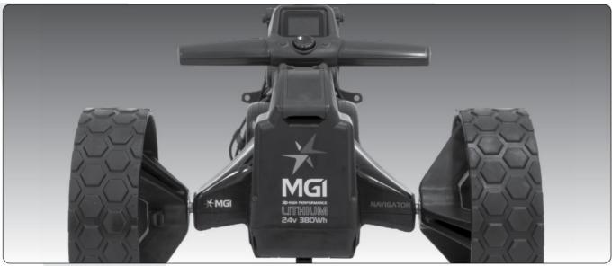
Press the grey release button on the wheel hub. Place the wheel onto the axle. You will need to match up the inner female groove on the axle and the male of the wheel. When placed in position simply release the button. You hear a "click" when the wheel is properly secured.
