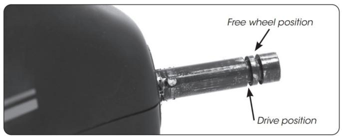
i. Drive position – Lock the wheel into the inner groove. To do so, press the black release toggle on the wheel hub, push the wheel onto the axle as far as possible and gently pull back until you hear a click. To test for drive position try rolling the wheel backwards. If you feel resistance then the wheel is now in drive position and ready to use. Repeat for both wheels.
