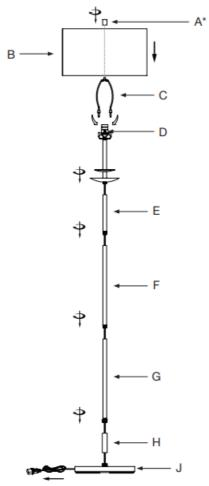
Carefully pull the power cord out from the Base (J) to remove slack.
