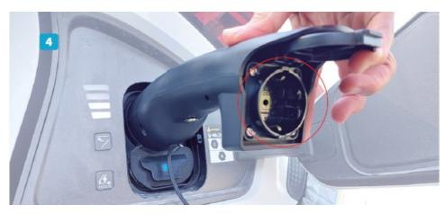
When you want to switch off the 230V power supply simply press the switch (2) again. To unplug the adapter from the vehicle you need to unlock it first by pressing the "unlock" button on the key fob (5).
