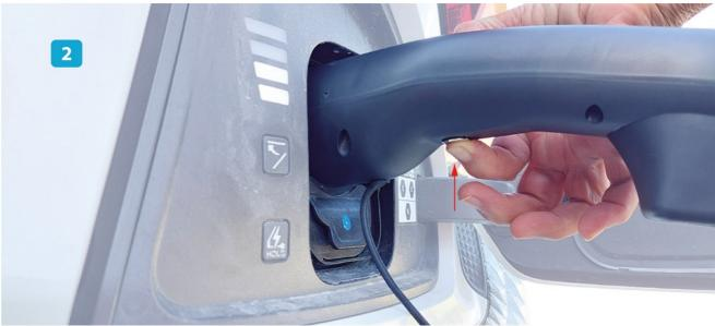
• The adapter will be locked in the car's socket and the LED indicator light will start glowing (3). When LED is on you have 230V AC mains electricity available at the socket (4) and you can now power various electrical devices.
