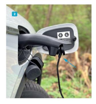
If the V2L-BY cuts-off power during use it may be due to an overload or low battery charge. Check the vehicle condition and charge level to determine why there is no output power.
