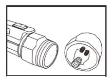
Cap with springs to align with the batteries.
