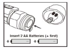
Observe correct polarity when installing batteries.
