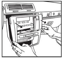
5. Remove (4) 9/32 screws securing the factory radio, disconnect the wiring, and then remove the radio.
