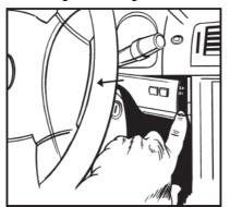
4. Using the panel removal tool, unclip and remove the trim panel surrounding the factory radio, including the climate controls.
