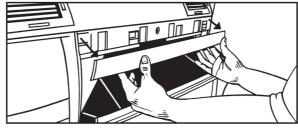
2. Unclip the upper edge of the panel below the steering column and let hang.
