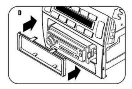
NOTE: To remove the radio unsnap and remove the ISO trim-plate. Using a flat blade screwdriver disengage ISO brackets from the radio housing and slide radio out of radio housing.
