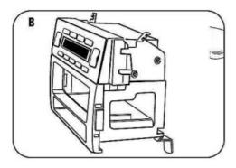
**3** Align the holes in the ISO brackets with the holes in the radio. Mount the brackets to the radio using screws supplied with the radio. (**Figure C**)
