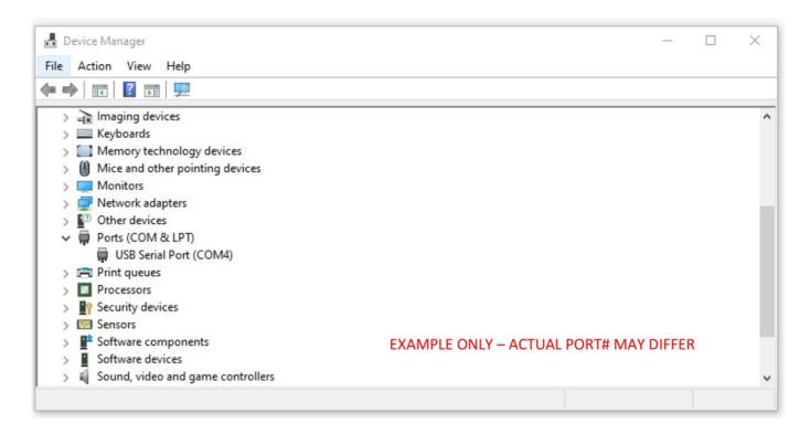
STEP 5: SELECT ACTIVE COM PORT# AND CONNECT TO CV-PS5200 USING PIC 32 Bootloader Application
