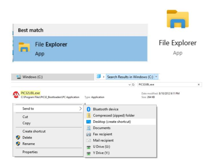
After extraction of CV5200r1\_xx.hex file (firmware update file) SECTION 1 for download, unzip files and application is completed. The application will now be available on the computer for future CV firmware updates (it is not necessary to re-install AN1388 Source Code 2014\_02\_14.exe application for future CV firmware updates).
