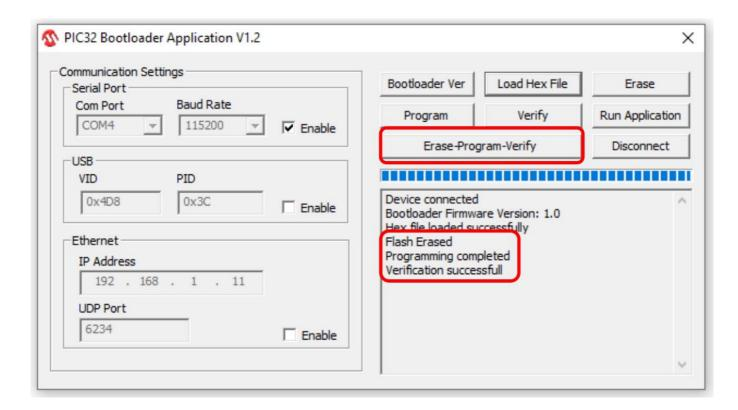
STEP 9: Press the DISCONNECT command button on PIC BOOTLOADER command screen
