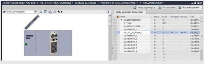
• First load the Controller project and connect the EB 80 to the associated IO-Link port.
