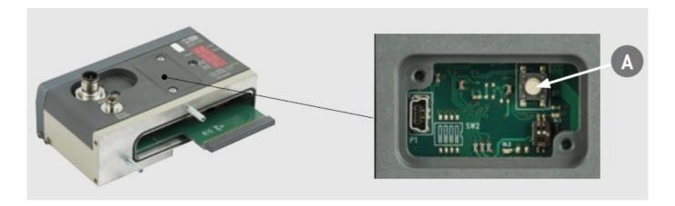
Connecting the EB 80 to the PC. Open the EB 80 Manager software.
