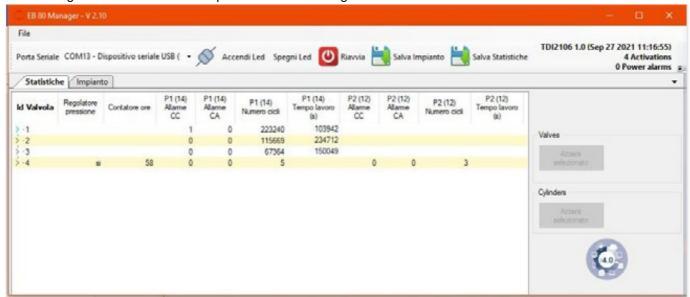
Select the serial port: COMx-MetalWork and connect up to the system by clicking on the connection icon. The data of all the valves, of pressure Regulators and configured actuators will be displayed.
