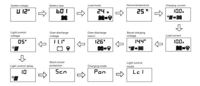
**Note:** The setting of boost charging voltage is applicable only in b04 and b07. When the battery voltage rises to this set voltage, PWM charging will be started. During normal charging, the arrow remains lit, and after entering the float charging, the arrow turns to flash slowly. Recommended to keep the default value.
