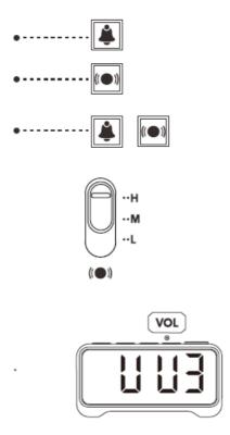
Set the Vibration Intensity Plug in the vibrator and slide the
